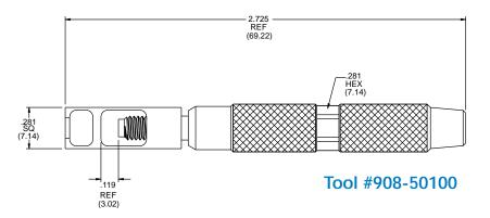
Universal tool for MicroMate (MMCX) right angle connectors for protective cap mounting and decoupling of connectors.
