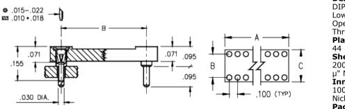
Description: DIP Dual In Line Socket Low Profile Solder Tail DIP Open Frame Through Hole Plating Code:
