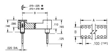
**Description:** DIP Dual In Line Socket Standard Solder Tail Closed Frame Through Hole Plating Code:
