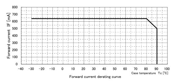
\*To keep case temperature lower than the rating, enough heat-radiation performance needs to be secured by using an adequate heat sink.
