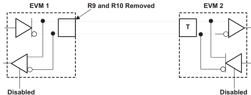
Figure 3. Point-to-Point Simplex Circuit
