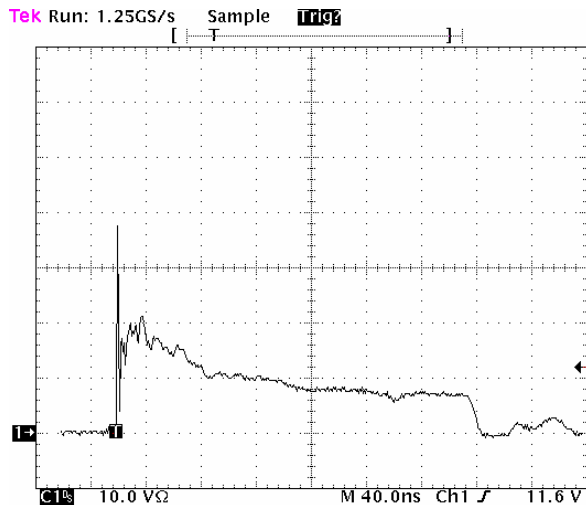
Figure 1. ESD Clamping Voltage Screenshot Positive 8 kV contact per IEC 61000-4-2
