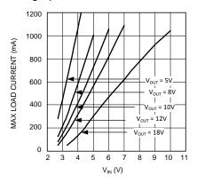
Figure 33. Max. Load Current (typ) vs V<sub>IN</sub> - "X"
