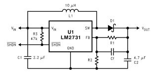
Figure 29. Basic Application Circuit
