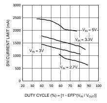
Figure 32. Switch Current Limit vs Duty Cycle - "Y"
