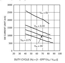
Figure 31. Switch Current Limit vs Duty Cycle - "X"
