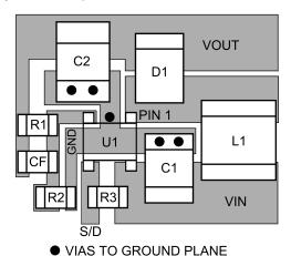
Figure 28. Recommended PCB Component Layout
