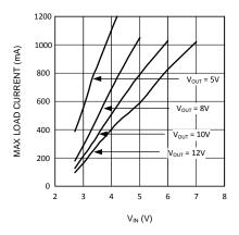
Figure 34. Max. Load Current (typ) vs V<sub>IN</sub> - "Y"
