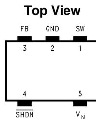
Figure 2. 5-Lead SOT-23 Package
