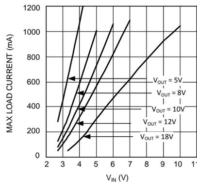
**Figure 33. Max. Load Current (typ) vs V<sub>IN</sub> - "X"**
