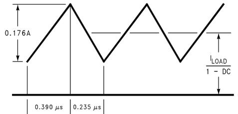
Figure 30. 10 μH Inductor Current, 5V–12V Boost (LM2731X)
