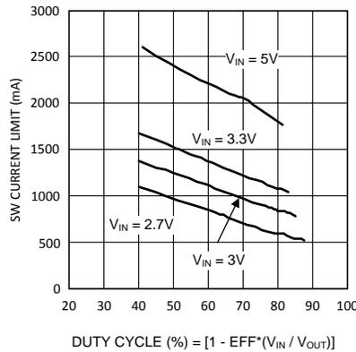
Figure 31. Switch Current Limit vs Duty Cycle - "X"
