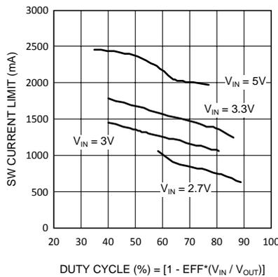
Figure 32. Switch Current Limit vs Duty Cycle - "Y"
