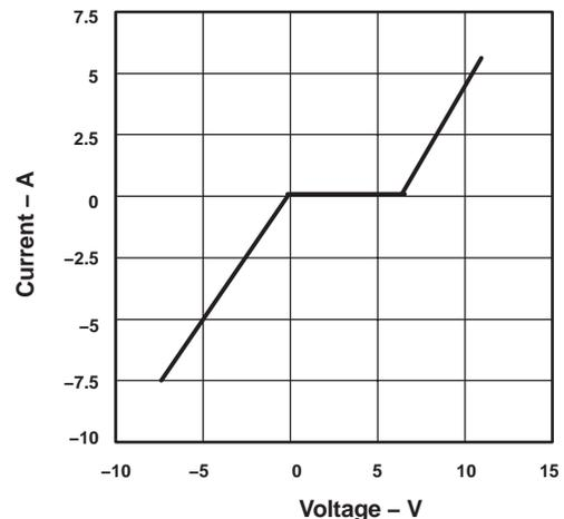
NOTE A: Typical current versus voltage curve was derived using the IEC 1.2/50- $\mu$ s surge waveform.
