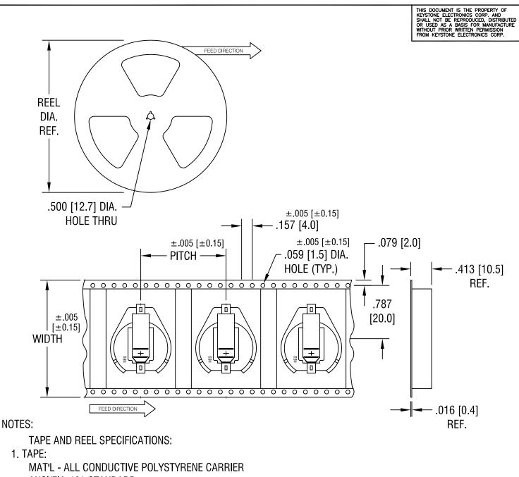
MAT'L - ALL CONDUCTIVE POLYSTYRENE CARRIER ANSI/EIA-481 STANDARD
