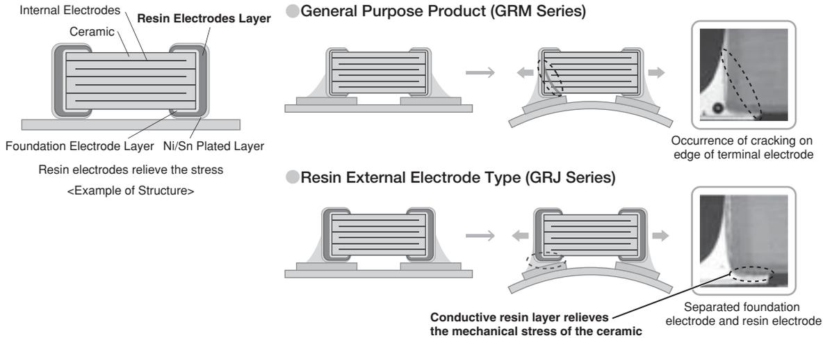
② Suppresses the occurrence of cracking caused by deflection stress at the time of board mounting, etc.
