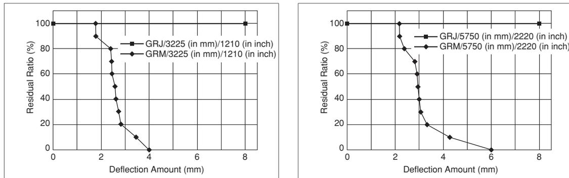
Due to the specification of the measuring instrument, measurements can be performed up to 8mm.
