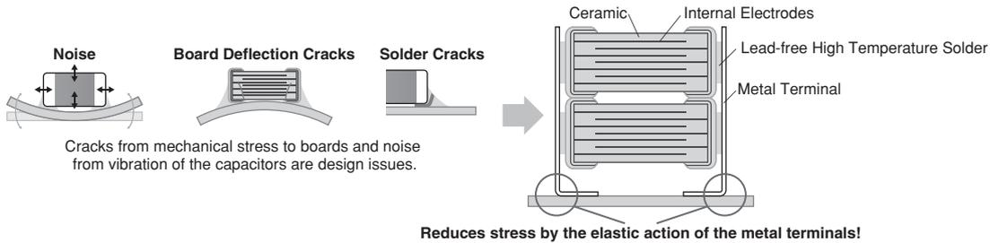
② **Substantially reduces noise, board deflection cracks and soldering cracks.**
