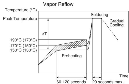
**[Allowable Reflow Soldering Temperature and Time]**
