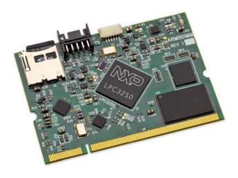
Modular ARM9 Microprocessor Plug-In System On Chip Module
