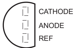
TLVH431 LP (TO-92/TO-226) PACKAGE (TOP VIEW)
