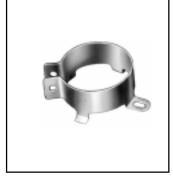
NACC VR mounting clamps may be used to mount any cylindrical capacitor with a 1" to 3" diameter that is to be mounted in a vertical position. Material is 1010 CRS, commercial grade #4 temper ASIscale. Parts are finished with .0001 (nominal) zinc chromate plating. Use for mounting CG types, PSU, HC/NP and MPD/MPF types. Material thickness is .035"
