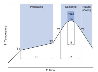
Preheating Soldering Peak Temp. Time Temp. Time Time Temp. T1 **T2** t1 Т3 t2 **T**4 t3 150°C 180°C 60 to 120s 10 to 30s 230°C 245°C 5s
