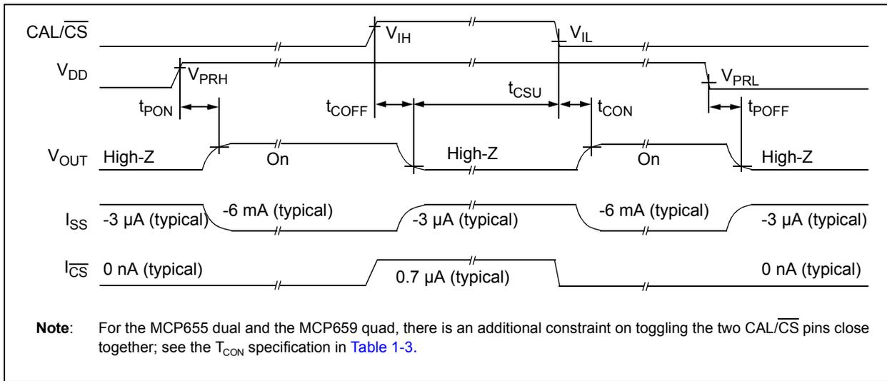
**FIGURE 1-1:** Timing Diagram.
