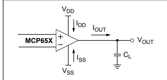
**FIGURE 4-8:** Diagram for Capacitive Load Power Calculations.
