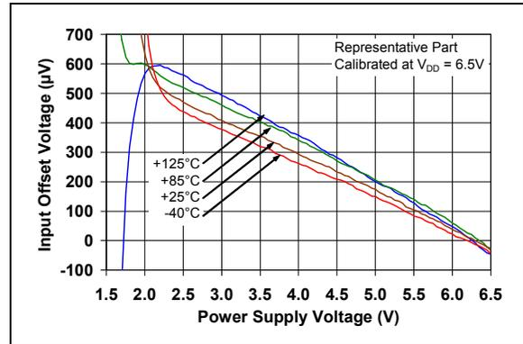
**FIGURE 2-4:** Input Offset Voltage vs. Power Supply Voltage.
