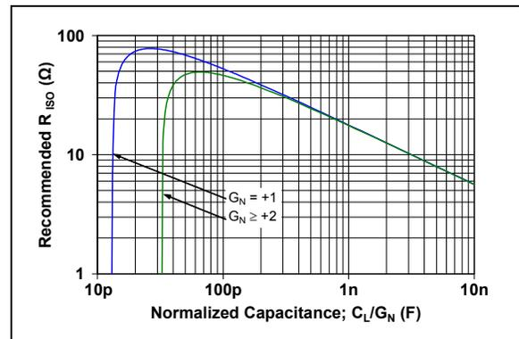
**FIGURE 4-10:** Recommended  $R_{ISO}$  Values for Capacitive Loads.
