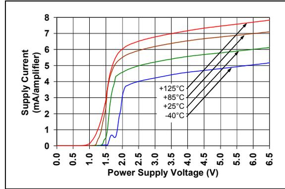
**FIGURE 2-19:** Supply Current vs. Power Supply Voltage.
