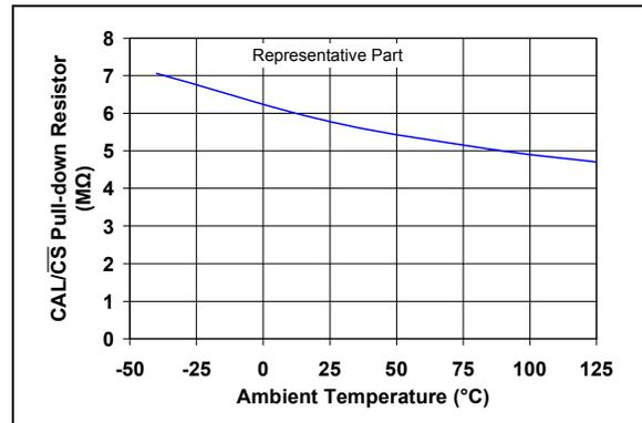
**FIGURE 2-49:** CAL/CS's Pull-down Resistor ( $R_{PD}$ ) vs. Ambient Temperature.
