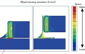
Stress load is concentrated on electrode section Use of metal cap reduces stress load on capacitor
