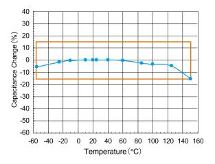
Electronic components for automotive use therefore must be able to withstand very high temperatures and be able to maintain stable operation over a wide temperature range. X7R and X8R type multilayer ceramic chip capacitors (high relative dielectric constant) fulfill these requirements.
