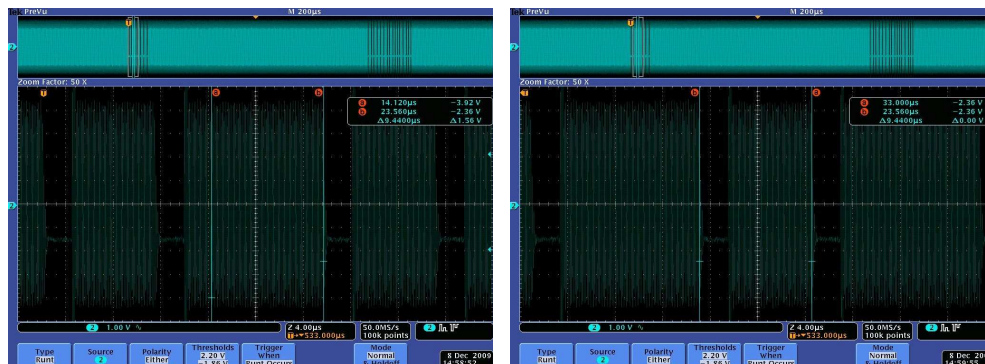
Figure 6-31. Receive Data Bits and Framing Level
