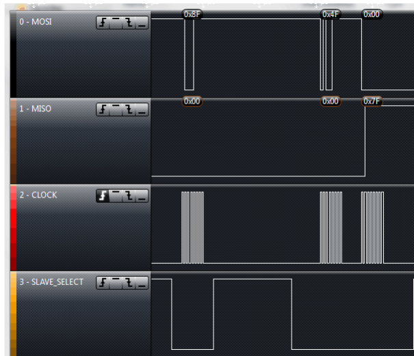
Figure 6-26. Reset FIFO and Read RSSI
