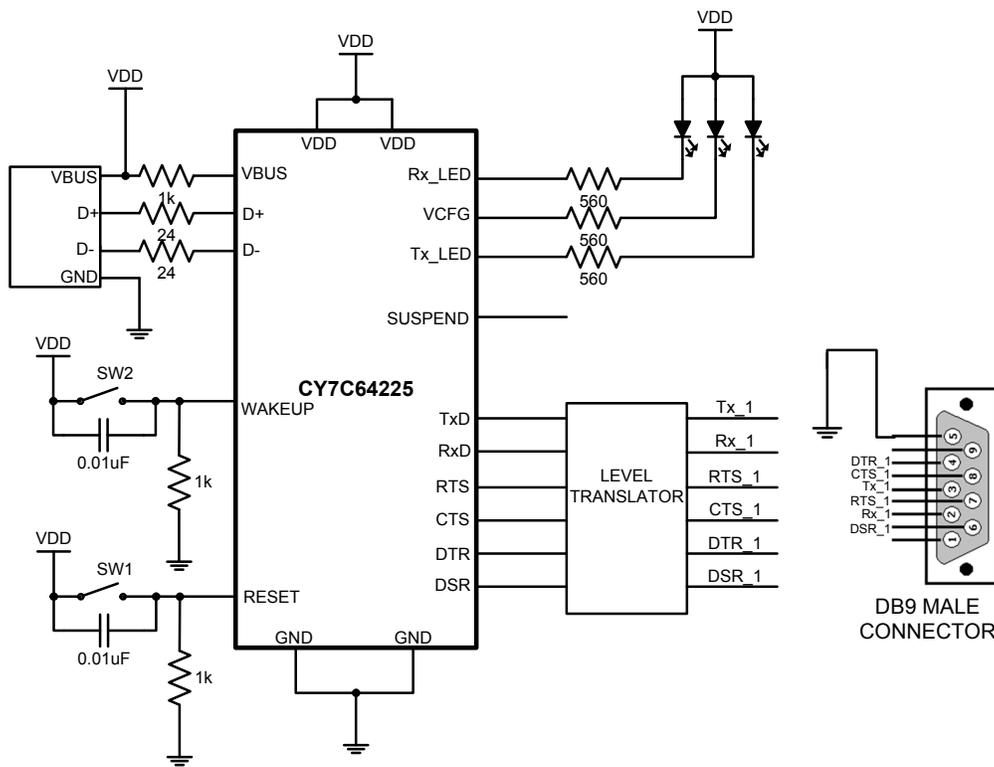
**USB to UART cable with TTL level UART signals**
