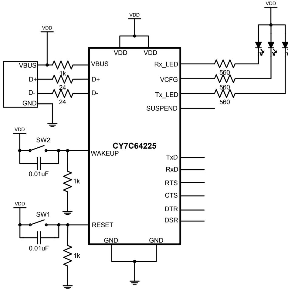
**Bus Powered Design using External Regulator**
