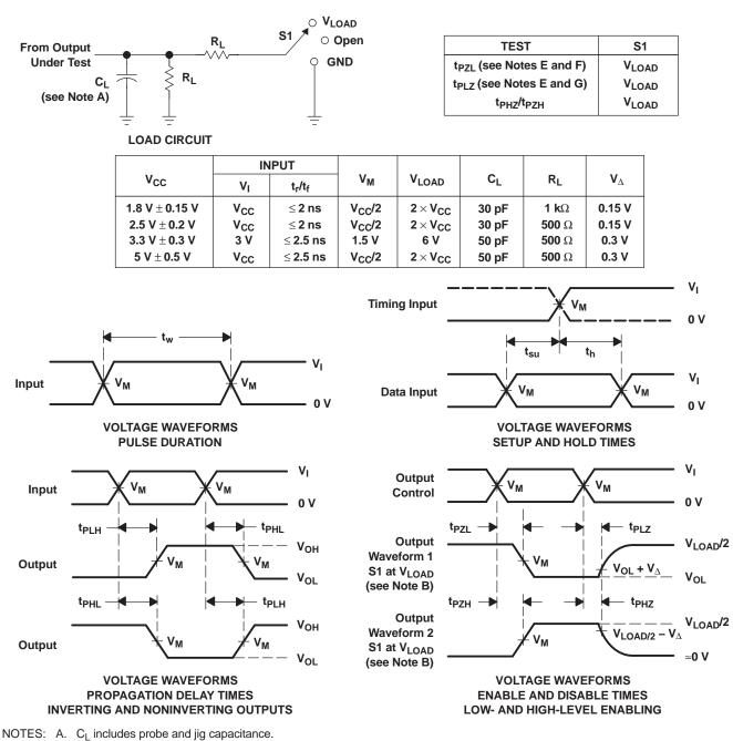
B. Waveform 1 is for an output with internal conditions such that the output is low, except when disabled by the output control.
