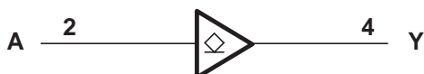
Logic Diagram (Positive Logic) (DBV, DCK, DRL, DSF, DRY, and YZP Package)
